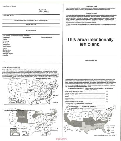
A Data Plate is affixed to each manufactured home. Typically located under kitchen sink, utility room, or master bedroom closet. The Data Plate provides information required for financing and installation.
