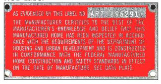
The Manufacturer Certification Label - a.k.a. HUD Label - is affixed to the exterior of each section of a manufactured home built on or after June 15, 1976. This label certifies compliance with HUD's Manufactured Housing Construction and Safety Standards.
